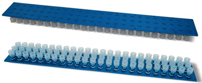
These suction plates provided with vacuum cups have been designed to ensure a better grip on uneven and very flexible surfaces (pasta or candy bags, blister or skin-film packs, thin cardboard boxes, etc.), which are difficult to grip with suction plates coated with foam rubber.
